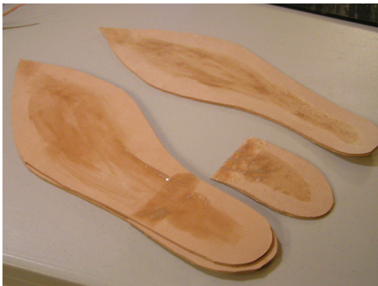
Heel Lifts Being Added to the Layers
